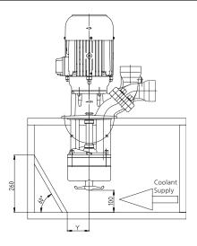
The SFC series cutter pumps are capable of cutting aluminum chips and similar materials and pumping of these materials along with the coolant fluid. An agitator located at the pump suction helps to break up and separate any large bundles of chips or birds nests which reach the pump suction.
