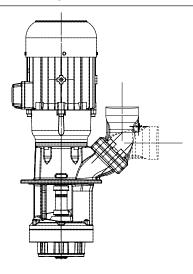
The cutter pumps of the series SPC are designed to handle and reliably cut long, stringy plastic chips.
