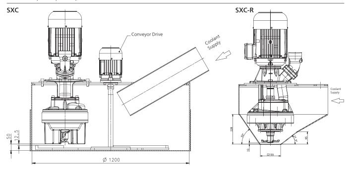
The cutter pumps of the series SXC are designed to handle low alloyed steels, machining steel (SXC-H) and cast iron / aluminum combinations (SXC). Chips can also be in the shape of birds nests or chip bundles.
