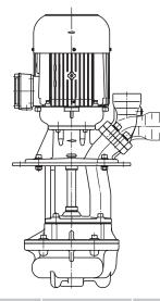
Vortex pumps are traditional lift pumps with a recessed impeller that allows for a sphere passage of up 50 mm. In order to ensure stable operating conditions the impeller must be fully flooded, and the pump must lift the fluid at least 3 - 8 m above the pump discharge.
