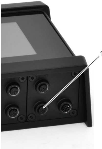
Fig. 11: Modbus RTU connection
